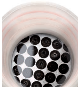
Testing the watertightness on the setting head side under 30 mm water column during 60 minutes
